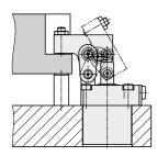
The **compact clamp** is a double-acting pulltype cylinder where a part of the linear stroke is used to swing the clamping lever onto the workpiece. The piston pull force is directly converted to clamping force less the friction losses.
